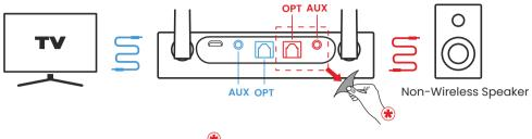
$<sup>^{</sup>igotimes}$ Remove the sticker to expose the **RX** ports.
