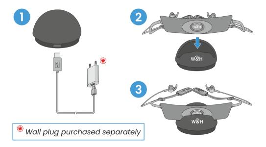
The LED indicator is red during charging and turns green when the headset is fully charged, typically within 2-3 hours.
