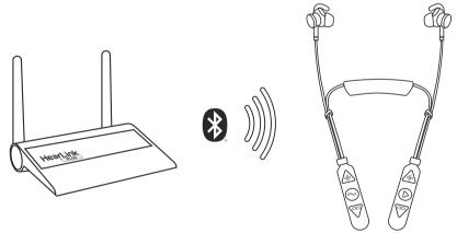
When pairing is complete (after 5-30 seconds) X will be illuminated on the HearLink PLUS panel.
